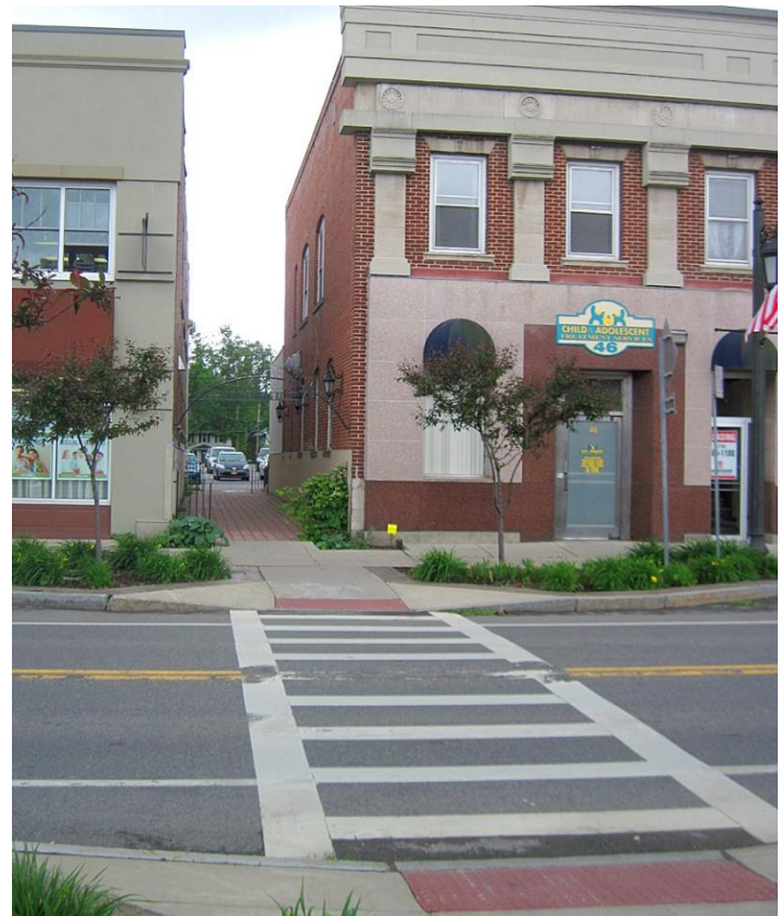
Figure 32.04.03-A: Mid-block connection example.
